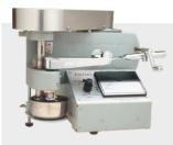
The lubricity test is designed to simulate the torque and drag produced by a given drilling fluid down-hole.
