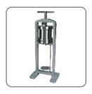
Filtration: Measuring the filtration behavior and wall-cake-building characteristics of a fluid are fundamental to the treatment and control of a drilling mud, no matter what the industry.
